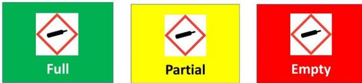
Empty cylinders must be stored in a room separate from the storage room used for full and partial cylinders.
