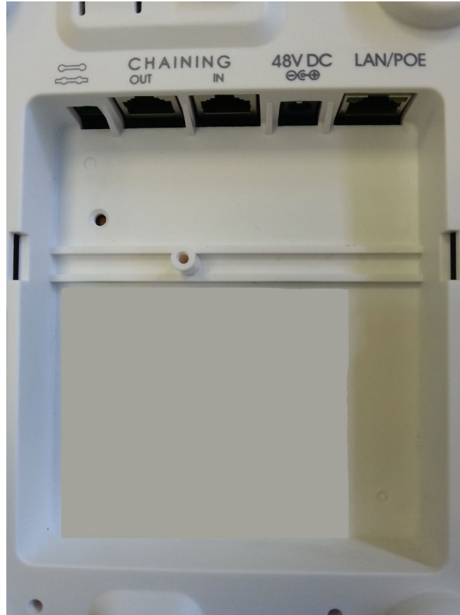
Figure 4: EX5200 Connector Wiring
