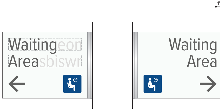
Two Line Layout with Symbol - Side A Maximum Characters Allowed: Approximately 10 per line
