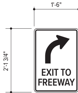
(B) Exit To Freeway
