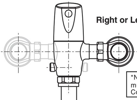
\*Note: The Critical Line (-C-L) on Vacuum Breaker must typically be 6" min. (152mm) above fixture. Consult Codes for details.
