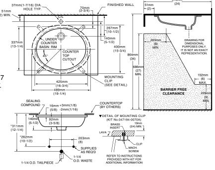
For Universal Design Options, top of counter may be mounted at 813mm (32") minimum from finished floor to meet ADA and ANSI A117.1 requirements. A 838mm (33") minimum mounting height is required for Ontario. Check local codes for heights and faucet handles requirements.
