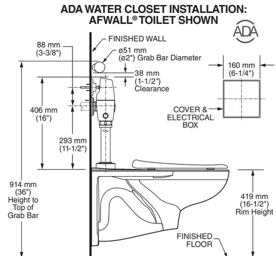
\*\* Flush Valve can be installed to meet ADA 2010 Section 609 when installed as shown
