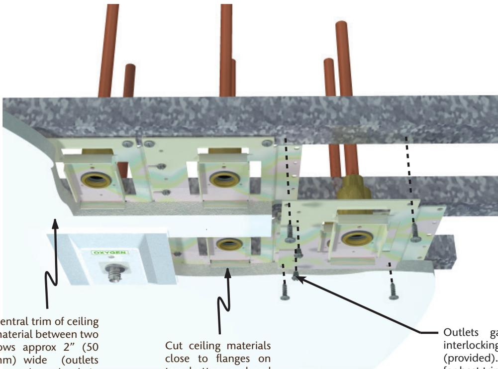
Use 1 1/4" (32mm) square or "U" channel for support. Brace solidly or suspend from deck. Space parallel rows 5 3/4" (146 mm) centerline to centerline. Outlet plates must be secured to supports top and bottom (4 places).
