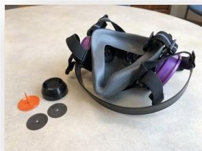
There are 2 black inhalation valves located on the inside of the respirator and one orange exhalation valve located on the outside of the respirator.
