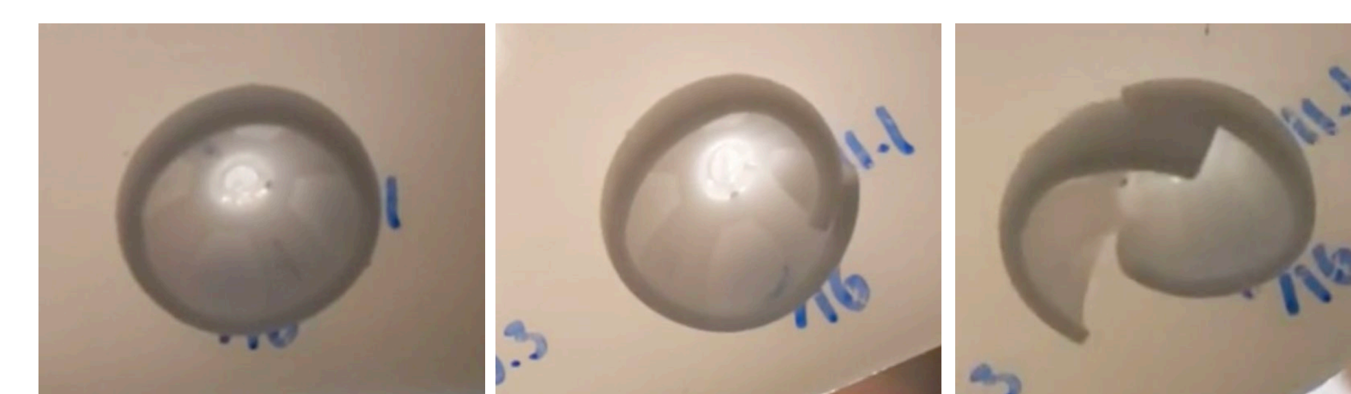
Figure 3. Images depicting gastrostomy tube mushroom retention discs with no incisions, one axial incision, and two axial incisions.
