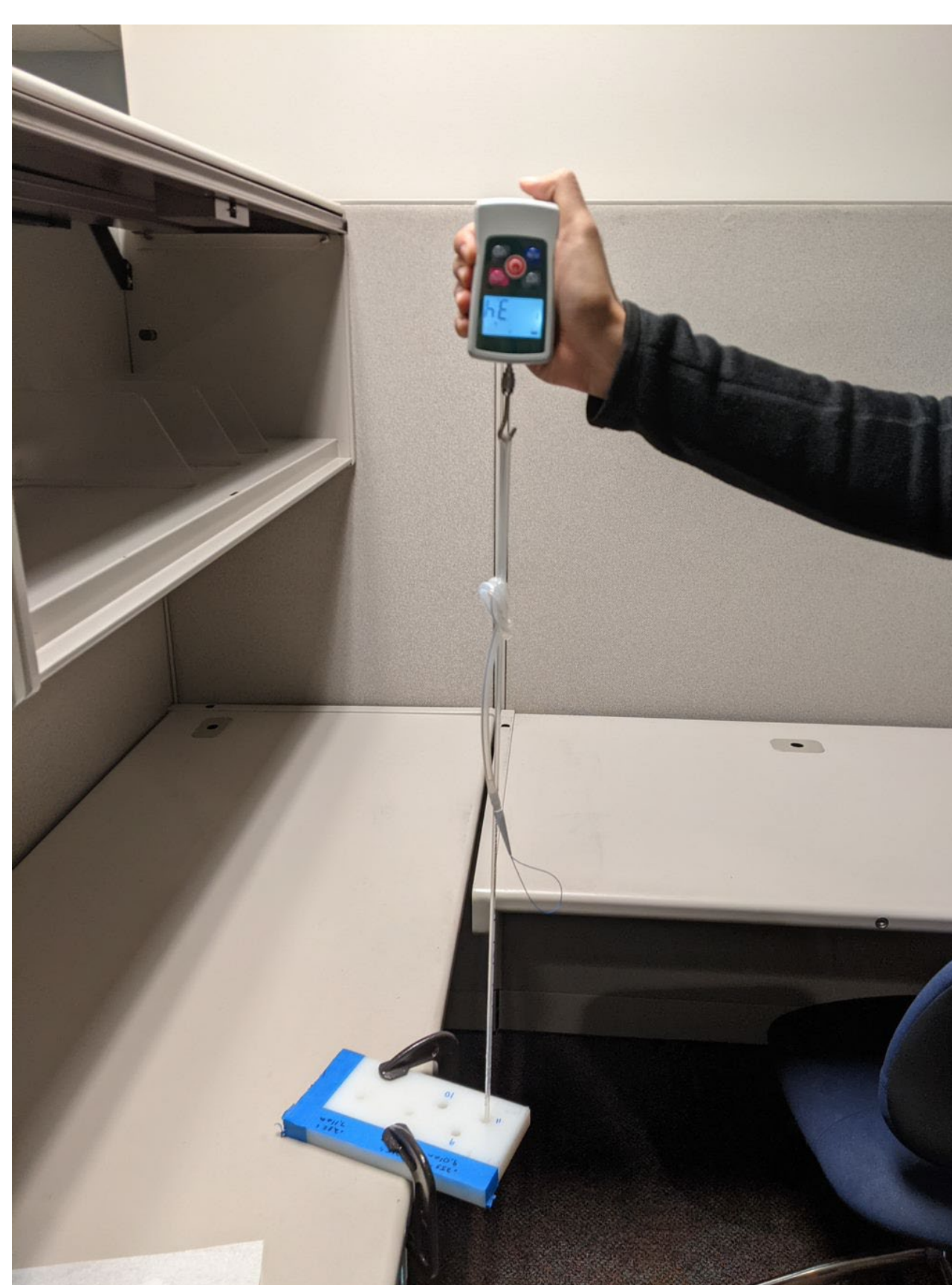
Figure 1. A secured polyethylene plate through which a mushroom-retained gastrostomy tube is pulled, attached to a digital force sensor
